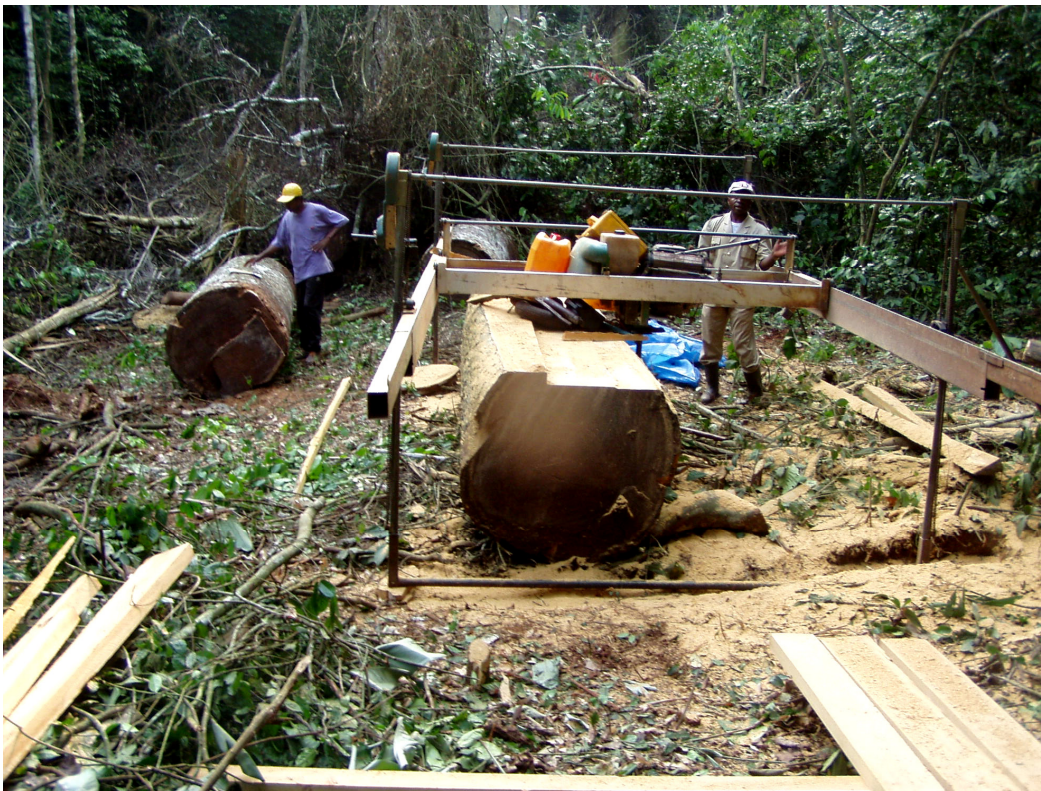
Photo: Felling and sawing site of an iroko
