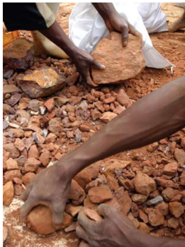
Congolese miners bag raw chunks of cassiterite, the ore from which tin is produced. Tin from DRC is used in the manufacture of consumer electronics, packaging, and alloys.
