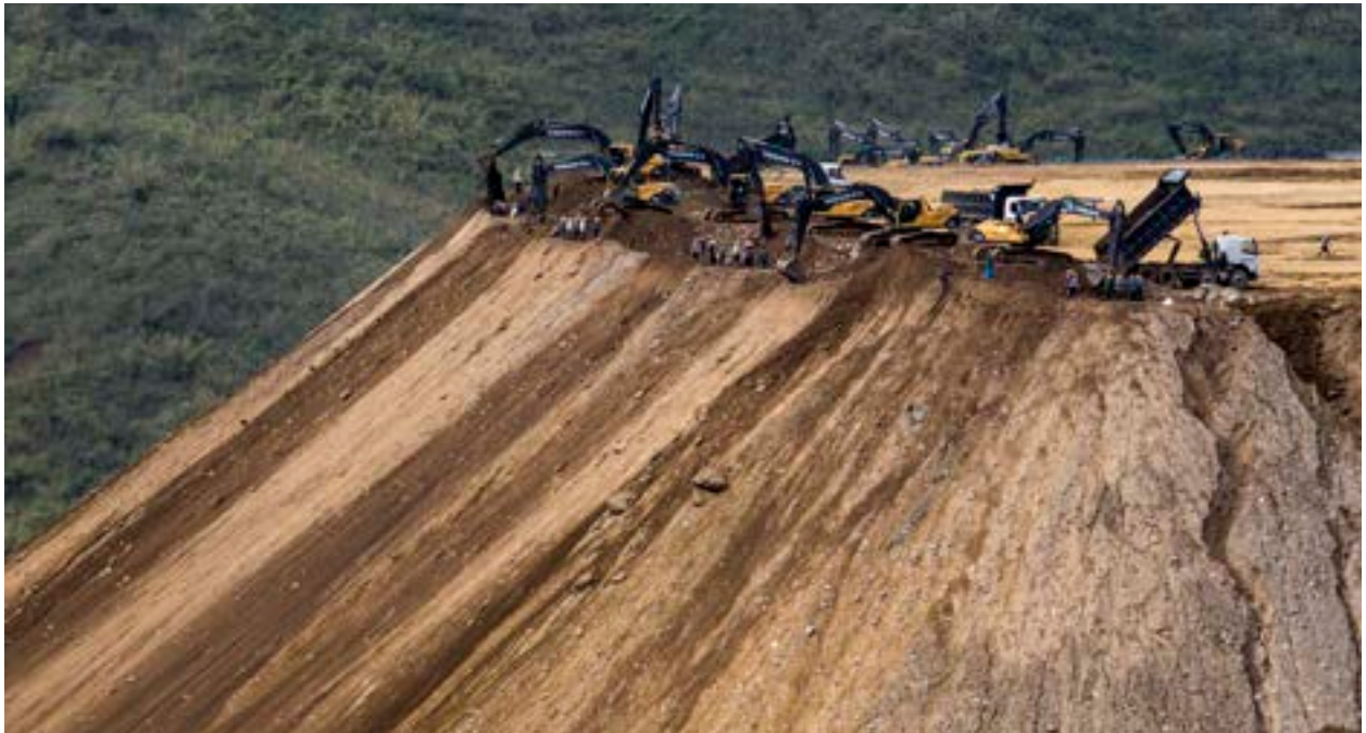
As companies ramp up mining activity, life-threatening landslides are increasingly common. At this site, at least 20 people were killed in January 2015 when heavy rains caused a waste dump collapse. CREDIT: Minzayar
