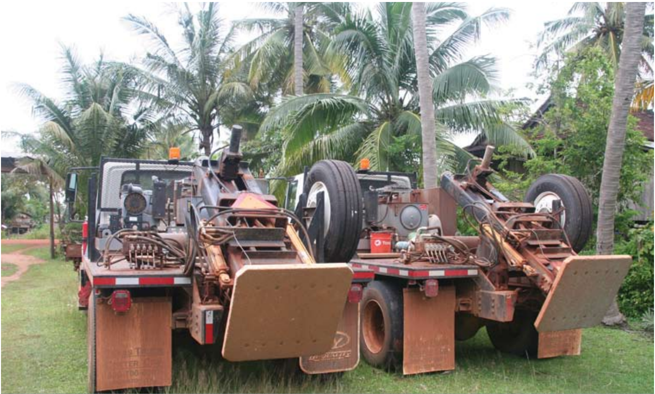
The testing involved laying out a 5 km-long tangle of wires alongside stretches of Highway 5 and the smaller roads running off the highway. Small sensors were inserted into the ground at intervals of 10-20 meters. Once the cables and sensors were in place, a ‘thumper’ mounted on the back of a small truck drove slowly along, stopping at each sensor to slam down a heavy square block. 384 This low-impact method provides data which will tell if there are petroleum reserves underground.
