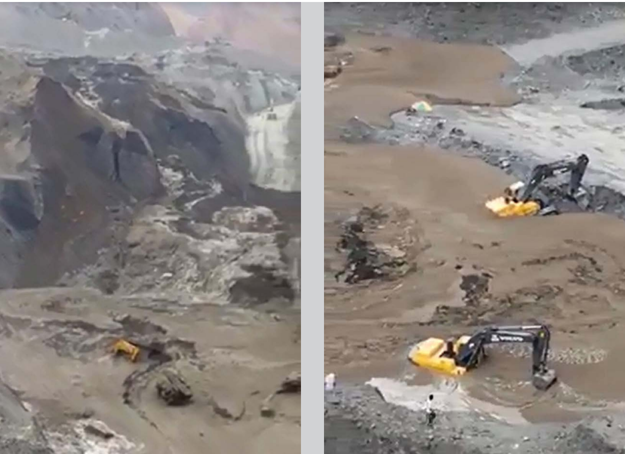
Stills from a video of a massive mud slide that took place at the Myat Yamon Kaday (#2) mine in April 2015. Local residents put the death toll at 30 to 60 people. The accident is said to have occurred due to the company's persistent dumping of tailings on a bed of liquid mud above the mine. The waste then shifted and flooded into the crater, engulfing workers and machines in its path.
