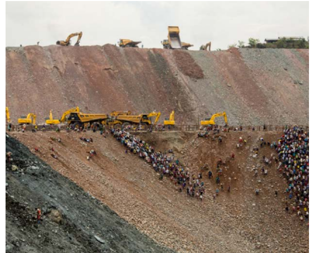
Dump trucks from the Myanmar Takaung company in Gwi Hka, Hpakant, tipping waste which jade hand pickers then search through. Myanmar Takaung and its associated companies have become very powerful players in Hpakant; controlling at least 50 mines. CREDIT: Minzayar
